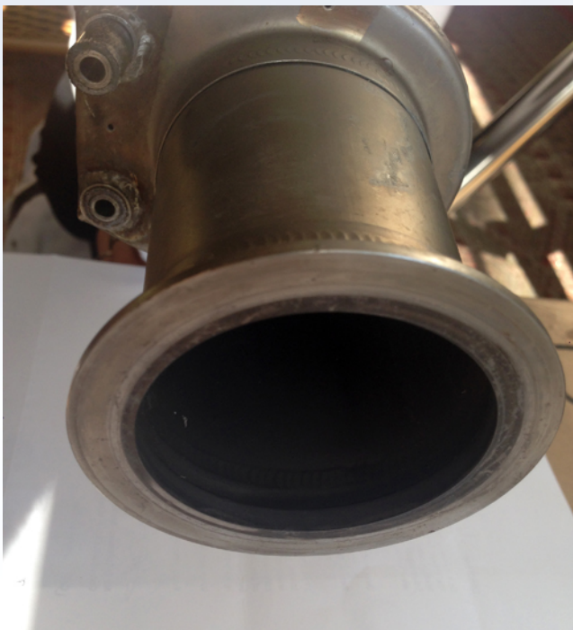
Bleed air off take port from a Boeing 737. Interior is black from oil contamination.
